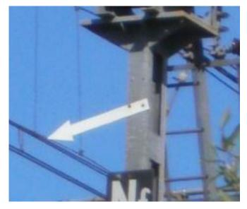
The white arrow is used to indicate which way the signal is addressed when it is implanted to its right (excluding Alsace and Moselle and outside ICS). In the case of the CSI, the contravene output signal must be arrowed.
