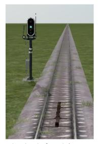
To choose which signal among the 8 possibilities that our basic signal can represent, we will use a device that exists in reality, and which is present necessarily before these signals: the crocodile. Each signal is preceded at 15-20 meters by a crocodile responsible for giving the driver the indication of a "closed signal" or "open signal".
